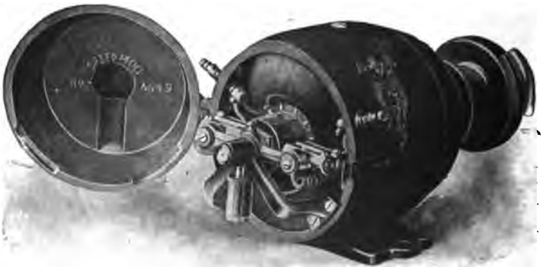
FIG. 342.—A Typical Ignition Dynamo—the Apple Dynamo Igniter. This shows the interior of the machine, the cover at the rear of the case being opened. The parts shown are the winding of one pole, the commutator brushes, the spider supporting the rotating spindle of the armature, and the wick-feed oil cup for lubricating the bearing of the spindle.
